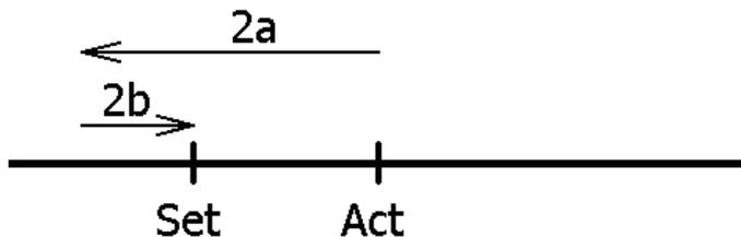
3. New setpoint position is only slightly larger than the current actual position and previously there was no positioning movement with loop (e.g. a manual movement):
