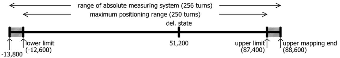
Here, the upper mapping end was decreased from the value 102,400 to 88,600. Consequently, a higher proportion of the possible positioning range is below 51,200 and a smaller proportion above 51,200.
