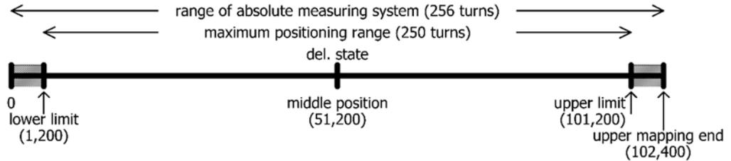
In the delivery state, the values from the following table result for the upper mapping end and the lower and upper limits:
