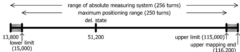
Here, the upper mapping end was increased from the value 102,400 to 116,200. Consequently, a higher proportion of the possible positioning range is above 51,200 and a smaller proportion below 51,200.
