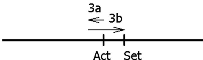
The maximum length of this distance is the loop length. If the setpoint differs from the current actual value by more than the loop length, it is approached directly.
