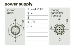
Supply voltage: 5-pin flanged Binder socket, model 763, no. 09-3441-xx-05
