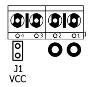
The former is generally selected if the motor power supply is run in a safety circuit with the EMERGENCY STOP and the databus has to remain active during an EMERGENCY STOP, or if the motor power supply does not permit correct operation of the bus adapter due to inadequate voltage stability or high interference voltages.
