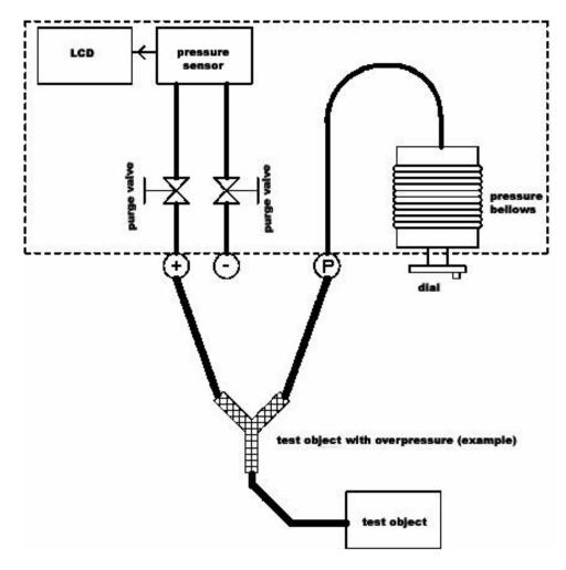
If the volume of the test object is high enough that the pressure bellows cannot generate enough pressure, use an additional manual pump (included with the calibrator upon request) and hook it up to the instrument with a Y connector.
