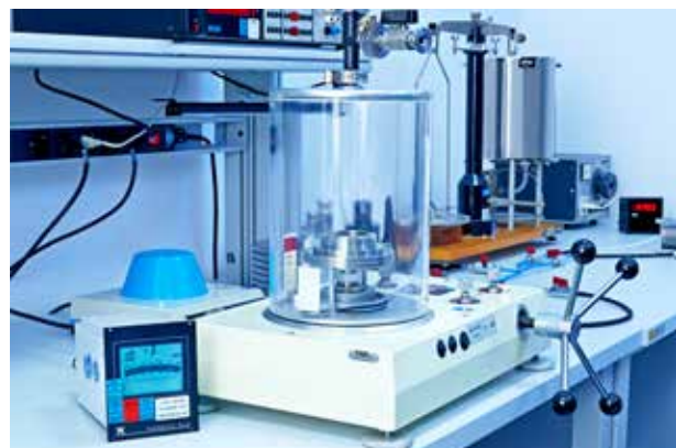
Piston manometer in the calibration laboratory of halstrup-walcher
