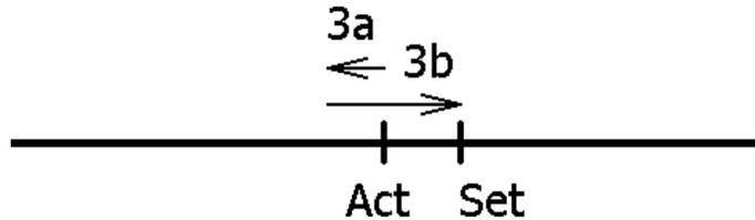
The maximum length of this distance is the loop length. If the setpoint differs from the current actual value by more than the loop length, it is approached directly.
