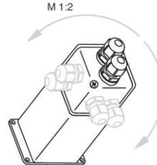
By turn of the cover around 90° are different positions of the cable glands possible
